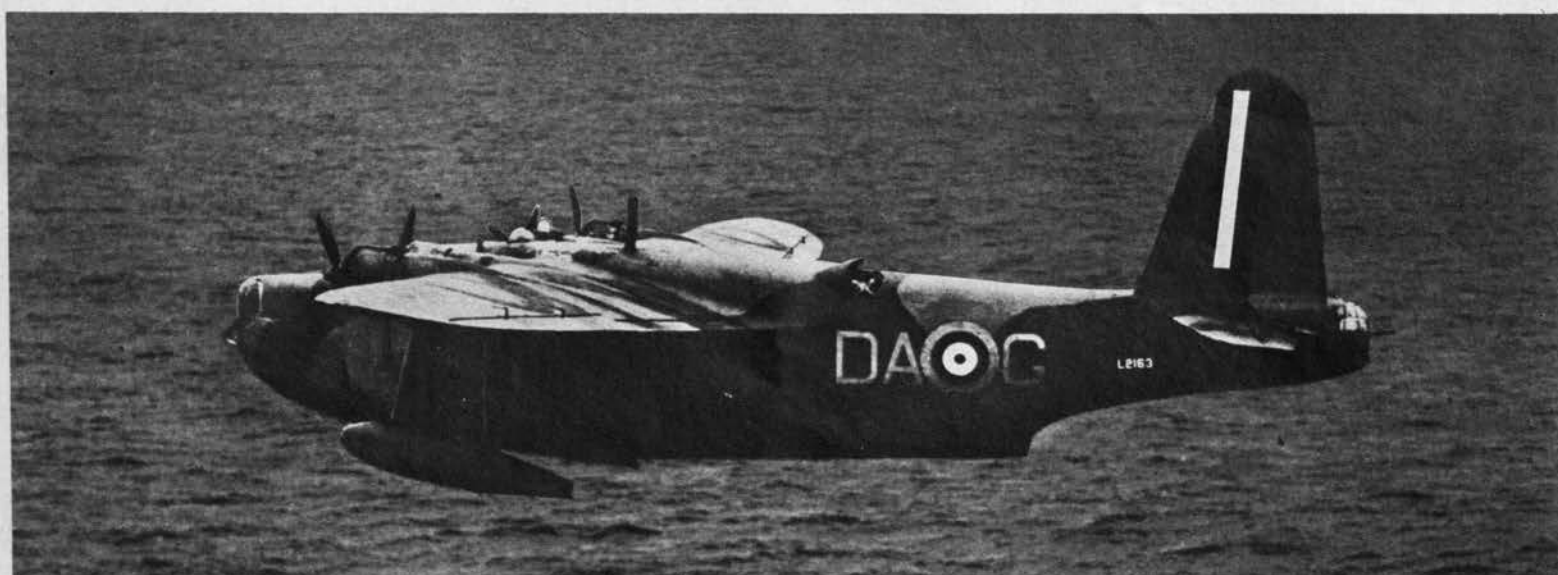
Fin and rudder on Britain's Sunderland are much taller than Emily's but not so wide. Nose is short and blunt and the hull has a decided
